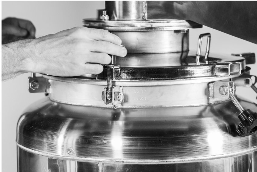
Figure 13: Operation of the thumb screws on the vessel.
