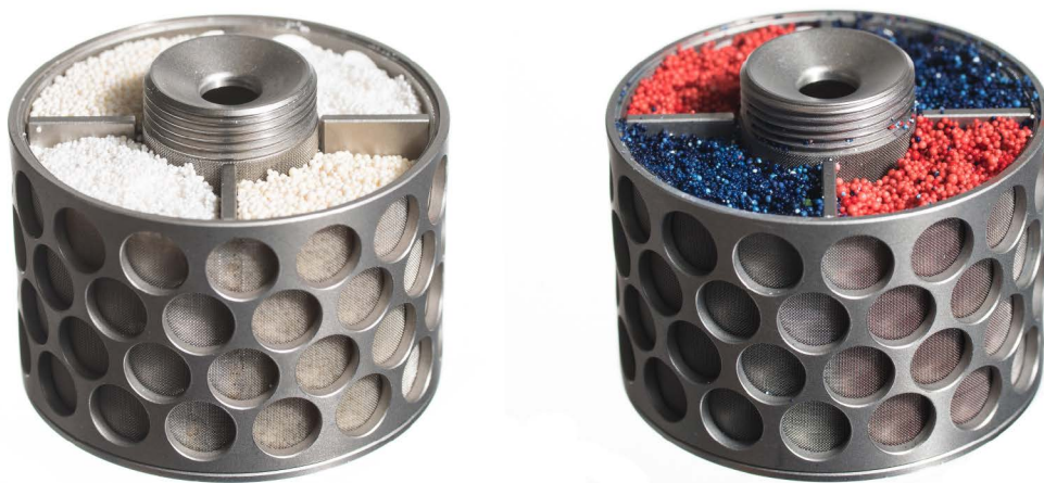
Figure 2. A SpinChem® rotating bed reactor (RBR) S2 packed with PuroLite® A500 Plus and Purosorb™ PAD700, before (left) and after (right) adsorbance of the two dyes.
