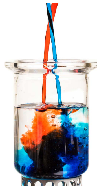
Figure 1. EasyMax™ 102 Advanced glass vessel filled with diluted Allura Red and Methylene blue solution.
