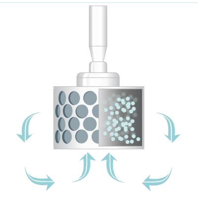
The SpinChem® RBR creates efficient mass transfer. The RBR aspirates solution from the bottom, percolates it through the bed of solid phase, and finally distributes it towards the vessel wall, thereby creating a continuous flow of solution.
