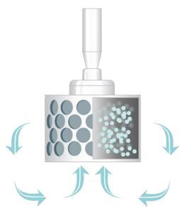
The SpinChem® RBR creates efficient mass transfer. The RBR aspirates solution from the bottom, percolates it through the bed of solid phase, and finally distributes it towards the vessel wall, thereby creating a continuous flow of solution.
