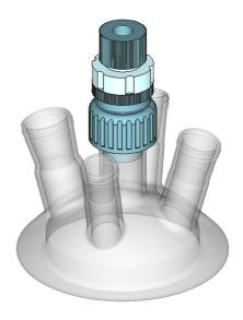
Pass RBR shaft through lid and shaft guide
