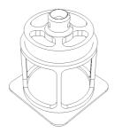
Fit bottom plate onto centre piece
