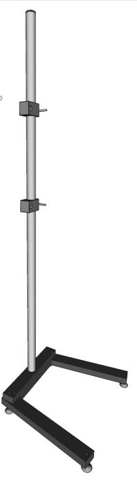
Fix bottom piece of vessel holder onto stand
