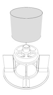
Make sure filter fits tight to bottom Complete seal of filter cannot be guaranteed
