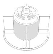
Fit filter inside outer ring Fold gently according to 6.1 & 6.2
