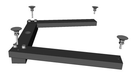
21 Attach screw handles to cross connectors
