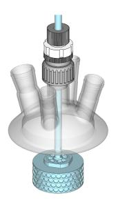
Place lid with shaft guide and RBR onto vessel
