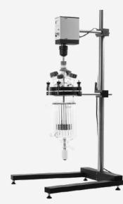
The quickest way to your rotating bed reactor experiments up and running. The all-inclusive kit allows processing of 250–1,500 mL volumes. Includes RBR S3, reaction vessel V3, lid, seal, hose connectors, shaft guide, holder, stand, and motor.
